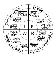
This chart shows four ways to figure each value: Amps (I), Volts (E), Ohms (R) or Watts (W).
